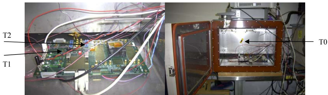
Figure 8: FPGA Evaluation board in the chamber; Figure 9: T0 thermocouple in the chamber.
