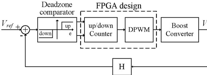
Fig. 2. Block diagram of the designed boost converter.
