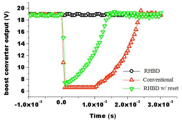
Fig. 5. Measured converter output transients after the injection of an error in both conventional and RHBD designs.
