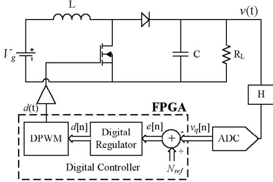
Fig. 1. Basic schematic of a digitally controlled boost converter.
