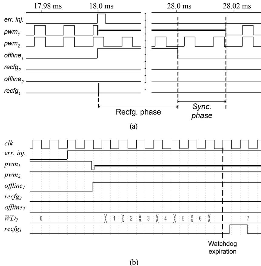
Fig. 6. (a) VHDL simulation of the overall system (b) Detail of the VHDL simulation, showing the expiration of the 3-bit watchdog timer of the FPGA2 after the occurrence of a SEFI on the FPGA1.
