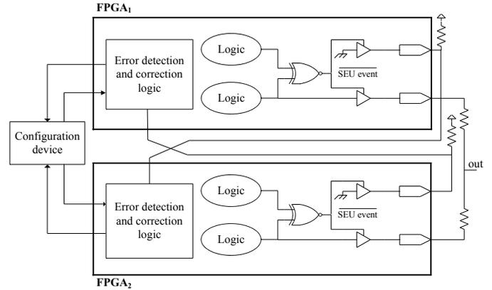
Fig. 3. Basic block diagram of the proposed RHBD technique. Two FPGAs, each of them containing two copies of the same design, are used to mitigate and correct SEFIs. The configuration device allows restoration of the correct configuration bitstream after the occurrence of an SEFI.
