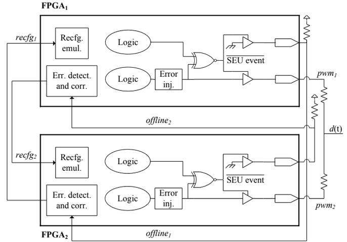
Fig. 4. Representation of the test-bed architecture of the digital controller. The configuration device has been replaced by the internal reconfiguration emulation (Recfg. emul.) block. The error injection module simulates the occurrence of an SEFI.
