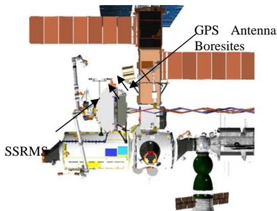
**Figure 14. SSRMS parked over GPS antenna array.**
