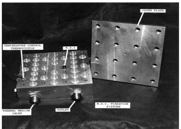
Figure 1. Fixture for NSI Thermal/Vibration Testing
