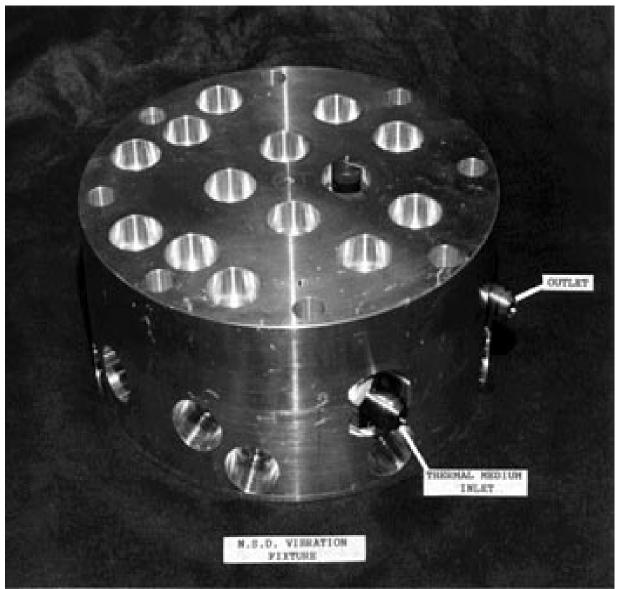
Figure 2. Fixture for NSD Thermal/Vibration Testing
