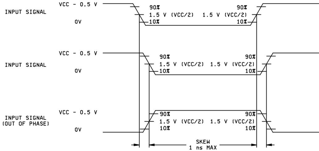
FIGURE 3024-2. Input waveforms.
