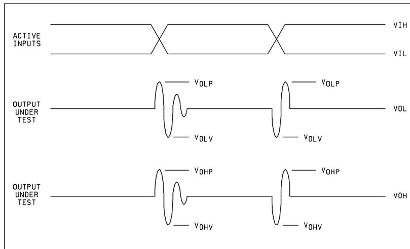
FIGURE 3024-3. Noise measurement technique.
