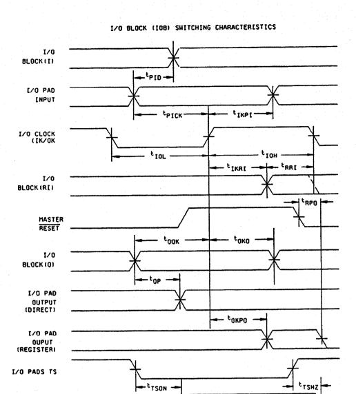
FIGURE 4. Timing diagrams and switching characteristics - Continued.
