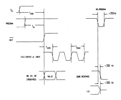
FIGURE 4. Timing diagrams and switching characteristics.
