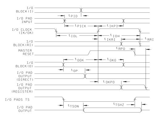
NOTE:  $t_{TSHZ}$  is determined when the output shifts 10 percent (of the output voltage swing) from  $V_{OL}$  level or  $V_{OH}$  level. See figure 5, circuit B herein for circuit used.  $t_{TSON}$  is measured at 0.5  $V_{CC}$  level with  $V_{IN} = 0.0 \text{ V}$  for three-state to active High, and  $V_{IN} = V_{CC}$  for three-state to active low. See figure 5, circuit A herein for circuit used.
