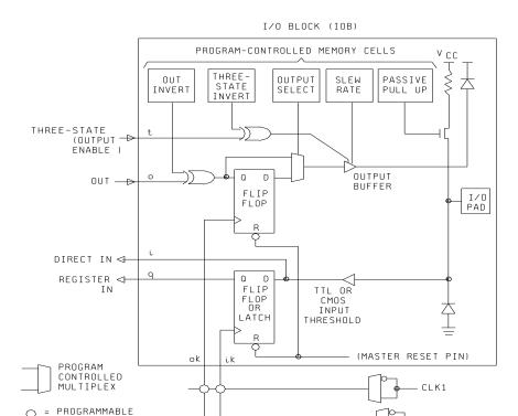
NOTE: The IOB includes input and output storage elements and I/O options selected by configuration memory cells. A choice of two clocks is available on each die edge. The polarity of each clock line (not each flip-flop or latch) is programmable. A clock line that triggers the flip-flop on the rising edge is an active low latch enable (latch transparent) signal and vice versa. Passive pull-up can only be enabled on inputs, not on outputs. All user inputs are programmed for TTL or CMOS thresholds.
