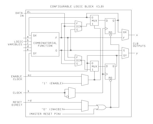
NOTE: Each CLB includes a combinatorial logic section, two flip-flops, and a program memory controlled multiplexer selection of function.
