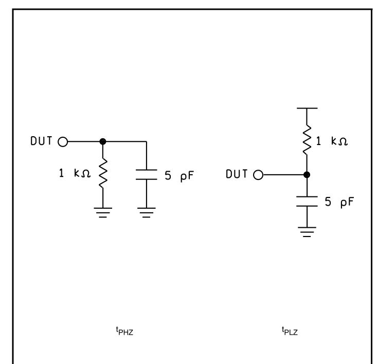
FIGURE 3. Output load circuits and test conditions.
