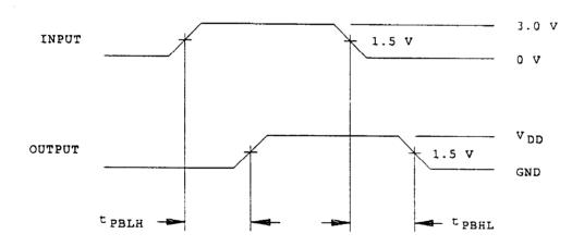
FIGURE 3. <u>Switching test circuit and waveforms</u>
