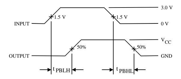
FIGURE 3. Switching test circuit and waveforms.
