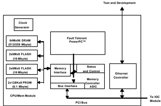
Figure 3. Block Diagram of CPU/Memory Section
