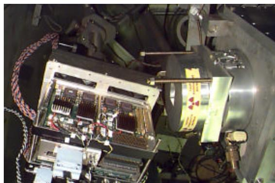
Figure 5. Picture of SEU Setup at Proton Beam
