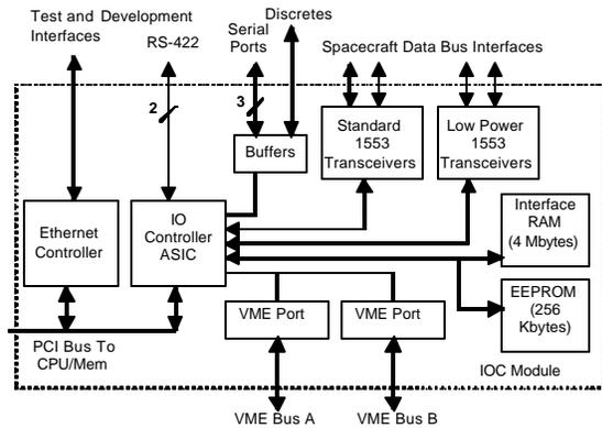
Figure 4. Block Diagram of I/O Section
